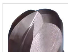
刃先形状 Cutting edge shape
